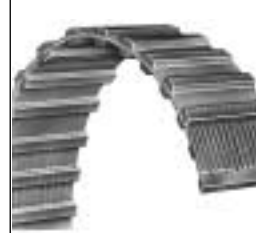
Synchro-Link® Double Sided Timing Belts (XL, L, H Rubber) (MXL, XL, T5, T10 Polyurethane) Designed for synchronized serpentine drives, these belts position teeth on both sides of the belt to provide smooth, precise performance under exacting drive conditions.
